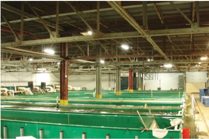
Figure 1. A warehouse/factory converted to Tilapia RAS production.
