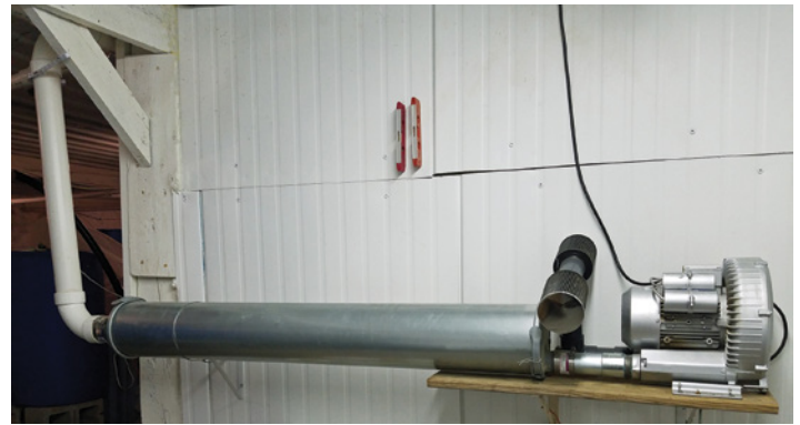
Figure 1. A regenerative blower with a cooling pipe. Two air filters prevent debris from entering the blower and should be examined regularly and cleaned if needed.
