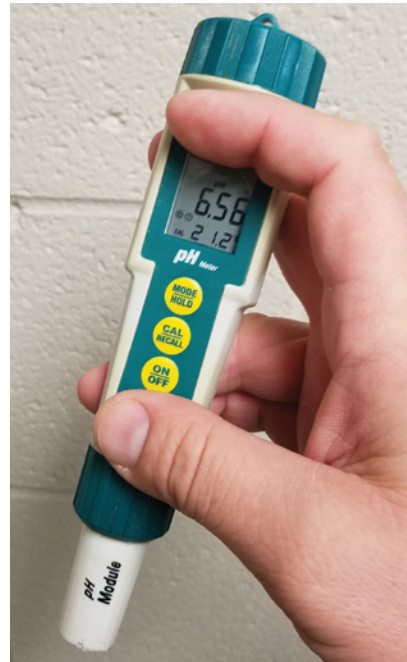
Figure 10. A pH and temperature meter. This type of meter is much less expensive than a multi-parameter style unit. Similar instruments can measure DO and salinity. Follow manufacturer's recommendations to calibrate all probes often; this ensures that they are accurate.
