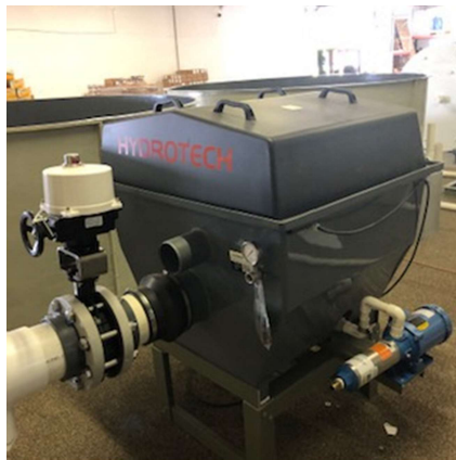
Skidded 801 Hydrotech Microscreen w/ high pressure pump ($700), and 6" actuated valve ($900) Sparus Pump with Constant Flow Technology
