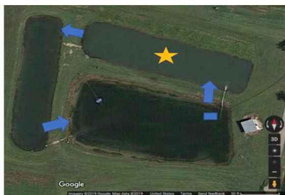
Figure 1. Aerial view of Brehm's Perch Farm. The fish pond is 0.25 ac (star) and the 2 waste treatment ponds total 0.75 ac. Water flow direction is indicated by arrows. The rectangle indicates the location of the two pumps used for circulating the water.
