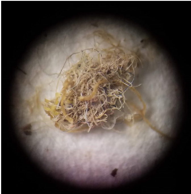
Tangled ball of microplastic fibers found in the digestive tract of a clam from Third Creek, Knoxville, Tennessee (25x magnification).
